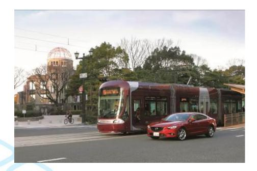
A first of its kind in the world, the system communicates using 700MHz radio waves, allowing cars and trams to share a variety of data, including the type and location of a vehicle, the direction they're heading, and braking and turn signal information. The ASV-5 sedan is equipped with autonomous millimetre wave and microwave sensors as well as cameras to monitor its surroundings and keep track of pedestrians, road markings, other vehicles and, of course, trams.
